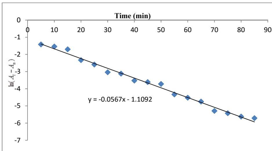
**Figure 1A:** Plot of  $\ln(A_t - A_\infty)$  versus Time (min) for the redox reaction of Malachite green and  $\text{NO}_2^-$  in aqueous solution,  $[\text{MG}^+] = 5.77 \times 10^{-5} \text{ mol / dm}^3$ ,  $[\text{NO}_2^-] = 6.41 \times 10^{-3} \text{ mol / dm}^3$ ,  $\text{MG}_{D_0}^+ = 0.208$ ,  $\lambda_{\text{max}} = 620 \text{ nm}$ , Temperature =  $25.0 \pm 0.1^\circ \text{ C}$ ,  $A_\infty = 0.065$ , Pseudo-first order rate constant,  $k_1 = 0.1306 \text{ s}^{-1}$
