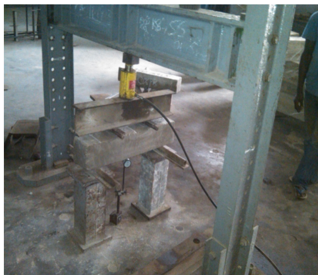
Figure 4: Experimental setup for the beam specimens
